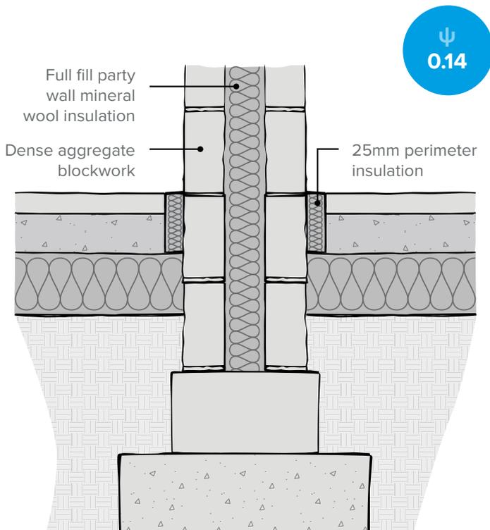
Use lightweight aggregate blockwork on the inner leaf to improve ground floor performance.
