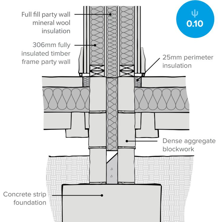
Use lightweight aggregate footing blockwork to improve ground floor performance.
