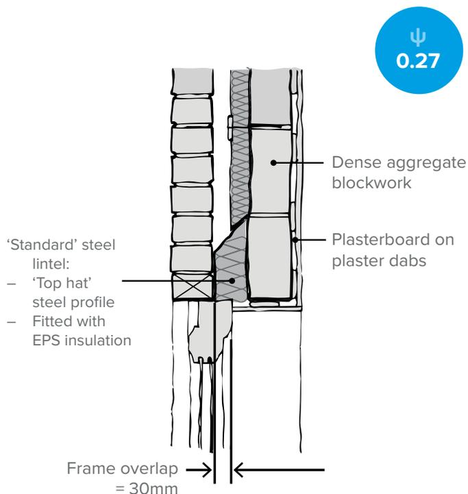
Use an insulated plasterboard reveal to improve performance for perforated steel lintels.
