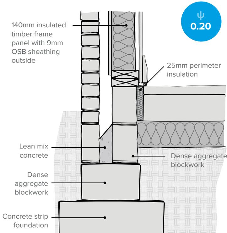
Increase the perimeter insulation thickness to improve ground floor performance.
