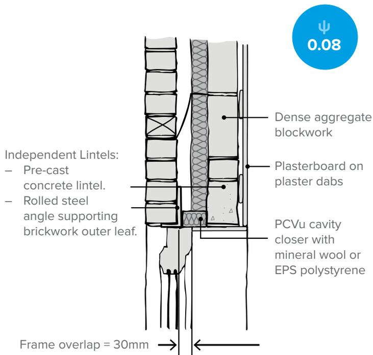
Use a cavity closer with a PU/PIR insulation core to improve performance for independent lintels.
