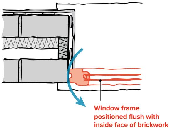
Window frame positioned flush with inside face of brickwork
