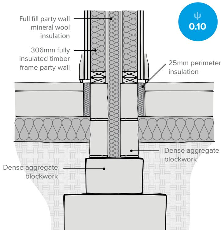
Use lightweight aggregate footing blockwork to improve ground floor performance.
