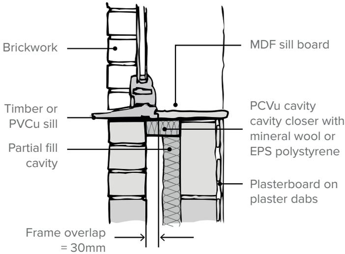
Use a cavity closer with a PU/PIR insulation core to improve the performance of sills and jambs.
